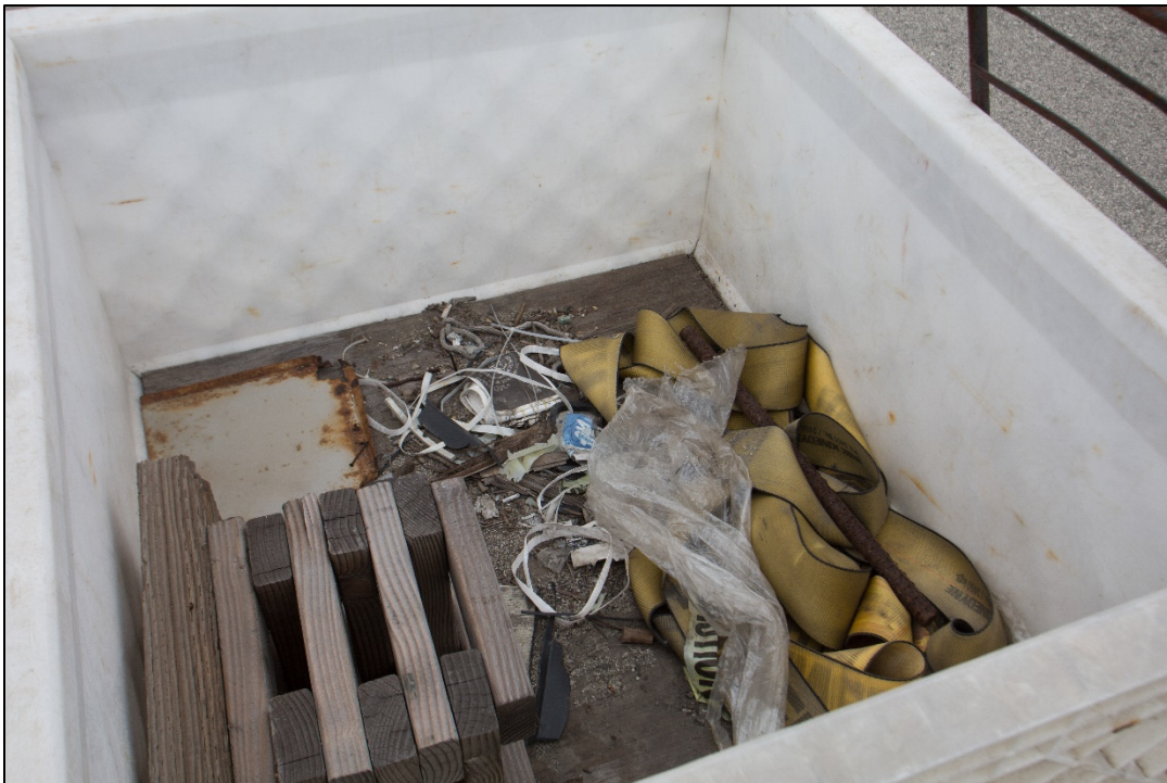
Figure 3-12. Collections of dirt and trash on equipment loaded on the barge. Equipment with piles of dirt should be treated as if harboring an invasive species and properly cleaned or removed from the barge shipment.
