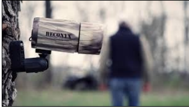
Figure 3-21. Equipment like Reconyx Microfire cameras are motion and infrared sensitive and should be used as part of a robust early detection and monitoring program to detect invasive species around barge facilities. Source: Reconyx.
