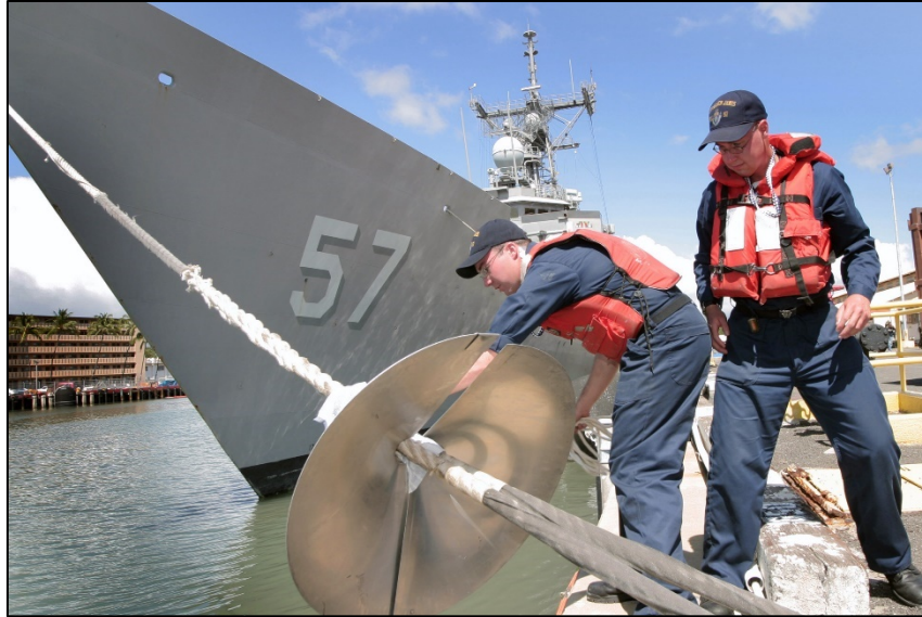
Figure 3-19. Example of a rat guard that should be installed on all vessels at dock travelling to NBVC SNI. Source: US Navy.
