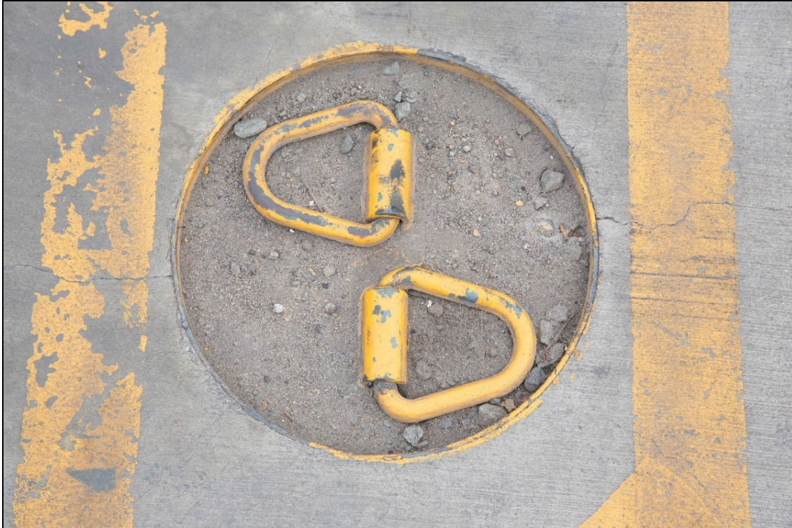
Figure 3-17. An example of a location where dirt can collect on barge decks. Barge decks must be pressure washed prior to loading.
