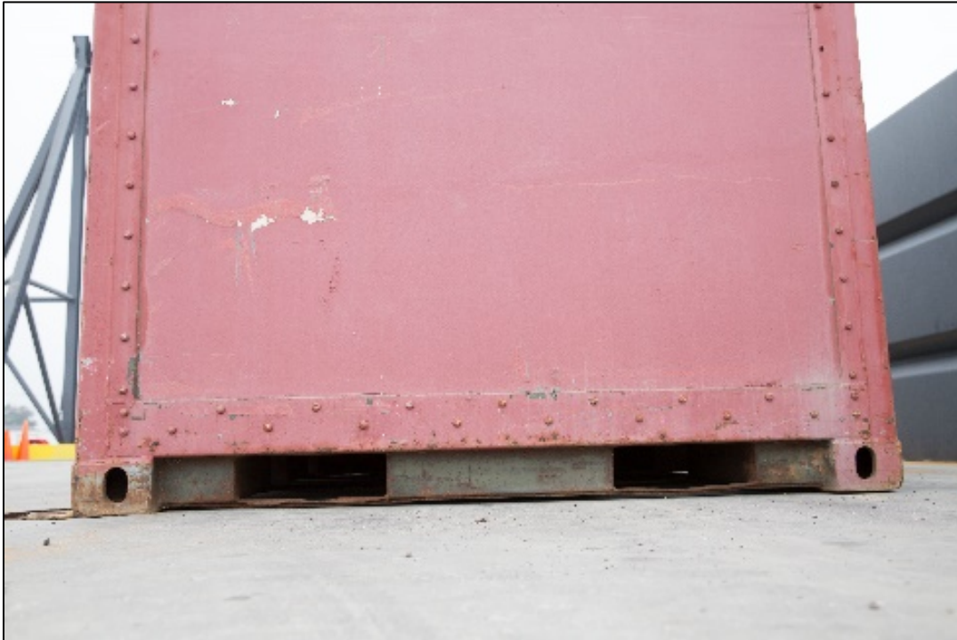
Figure 3-11. Fork lift holes should be inspected with flashlights to ensure no animal harborage prior to departure.
